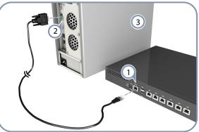
Connect a PC to the wireless controller console port using the included console cable.
