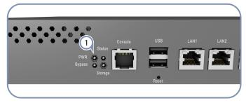
Verify basic wireless controller operation by checking the system LEDs. When operating normally, the PWR LED should be on green.
