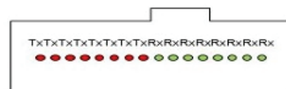
Figure 2 – 400GBASE-SR8 fiber interface variant 2
